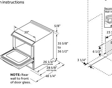
30 Side Wall 30" (see note) 0" minimum to cabinets above counter Recommended Wall-mounted 0" Right side Minimum 0" Left side to cabinets below Minimum cooktop to side wall 36 24 3 1/8" 30 **NOTE:** Minimum to bare cabinet above: see Installation Instructions for alternate installation configurations.
