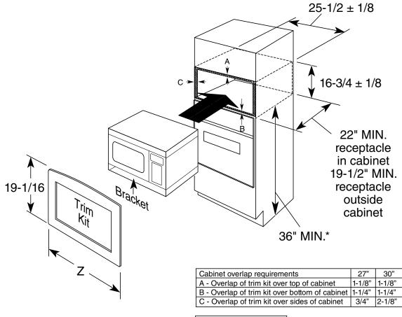
\*For ADA compliance, the microwave must be installed no higher than 36-1/4".
